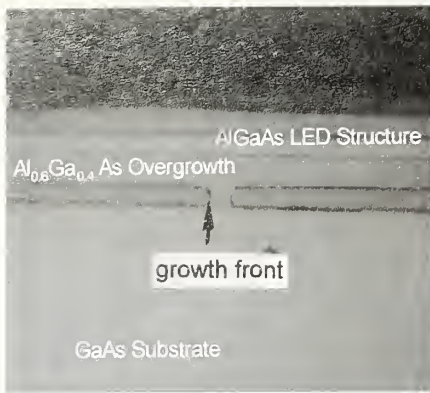
Cross-sectional photomicrograph of a light emitting diode showing device active layers and buried mirror overgrowth.
